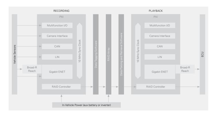
We typically deploy a PXI chassis in a vehicle and interface it to live camera, ultrasonic, vehicle bus, and environmental sensor data from typical driving situations. We use this live data to train and validate our computer vision deep learning algorithms at the bench later.
